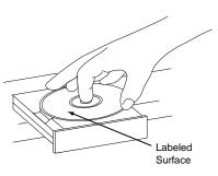
To close the drawer, press the appropriate Open/Close Button **G14 3 27** or gently press on the outside of the front cover of the disc tray. When the drawer is closed the word CLOSE will appear momentarily in the Time/Message Display **F**, and the letters TOC will begin to flash in the display once the drawer is completely closed.
